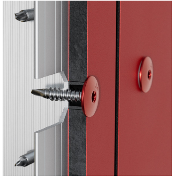
Detail view of sliding point for LT system classic
